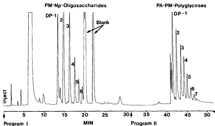
Figure 5. HPLC separation of mixture containing Np-derivatives (Fig. 1) and PA-PM-oligosaccharides obtained from corn syrup. Column: C-18 Spherisorb, 15 cm X 4.6 mm (ID). Program I, 40 to 100% acetonitrile:water (0.1 M Acetic acid), 1 ml/min, 30 min, recycled column to 40% acetonitrile:water (0.15 M ammonium hydroxide). Program II, 40 to 80% acetonitrile:water (0.15 M ammonium hydroxide), 1 ml/min, 20 min. Peaks not labeled are unidentified.
