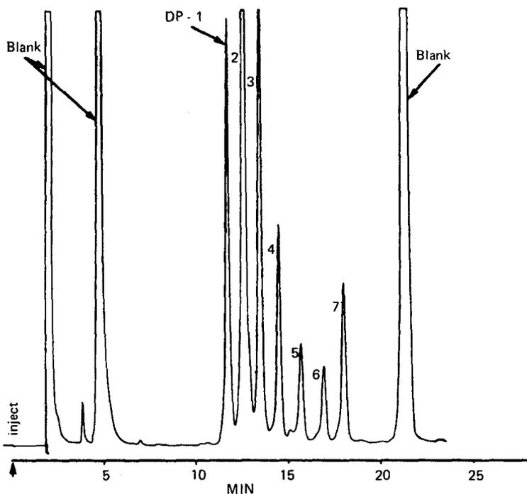
Figure 1. Mixture of naphthoylated products from partial reductive cleavage (4 minutes at 0°C) of permethylated  $\beta$ -cyclodextrin, approximately 0.01  $\mu$ g total material. Column: C-6 Spherisorb, 25 X 4.6 mm (ID). Elution solvent: 50% to 60% acetonitrile in water (0.15M ammonium hydroxide), 1 ml/min program 15 min. Peaks not labeled are unidentified.
