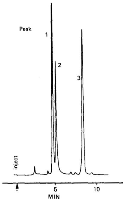
Figure 3. Products following reductive cleavage for 4 min at 0°C of PA-PM-maltotriose; reaction stopped with water; methylene chloride extract directly analyzed by HPLC. Column: C-6 Spherisorb, 25 X 4.6 mm (ID). Elution solvent: Acetonitrile:water 55:45 (0.15M ammonium hydroxide), 1 ml/min. Peaks not labeled are unidentified.
