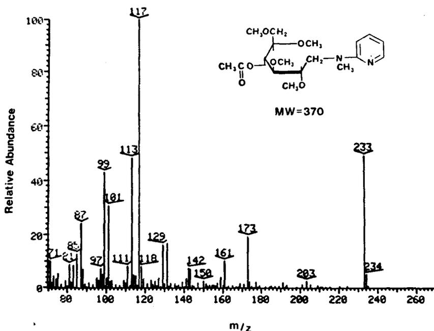
Figure 9. Electron ionization mass spectrum of peak 3 (Fig. 6); 1-(pyridinylmethylamine)-4-O-acetyl-2,3,6-O-methyl-D-glucositol.
