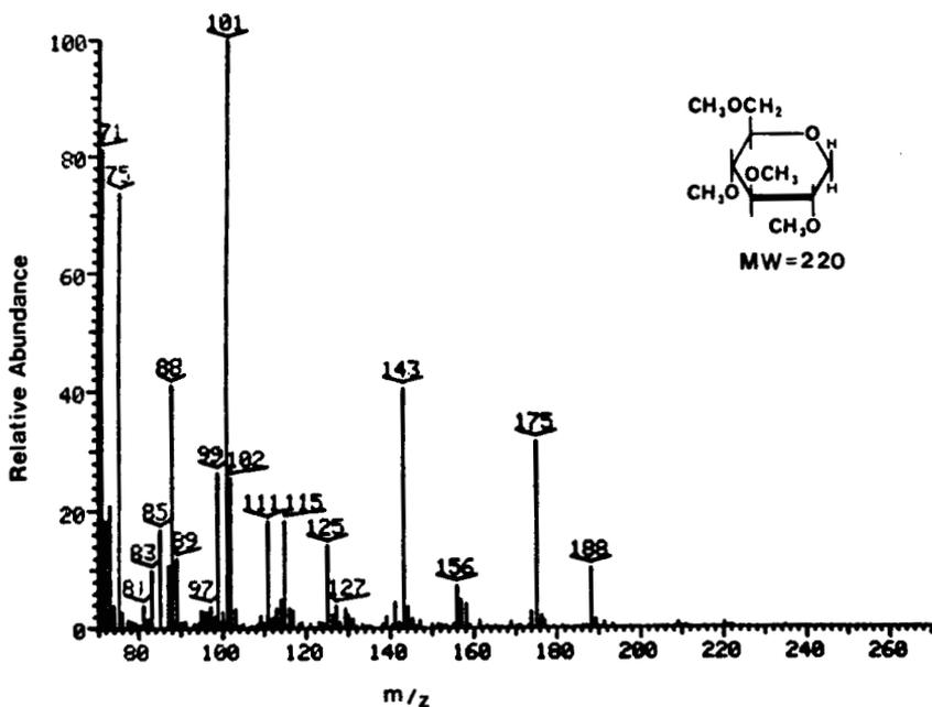
Figure 7. Electron ionization mass spectrum of peak 1 (Fig. 6); 1-deoxy-2,3,4,6-O-methyl-D-Glucopyranose.
