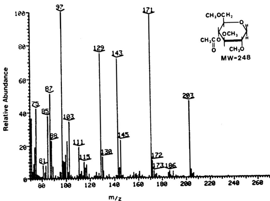
Figure 8. Electron ionization mass spectrum of peak 2 (Fig. 6); 1-deoxy-4-O-acetyl-2,3,6-O-methyl-D-Glucopyranose.
