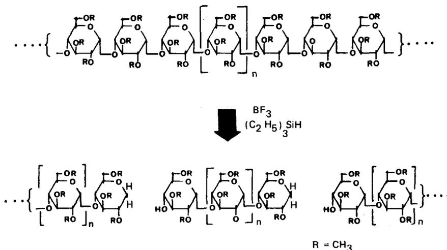
Scheme 1. Generalized accounting of partial reductive cleavage on linear glucopolymer. The oligomeric series will consist of three different series (i.e., terminal, reducing and intermediate).
