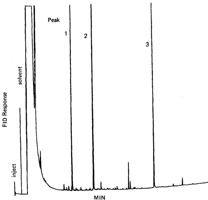
Figure 6. Gas-liquid chromatography of products obtained following two hours reductive cleavage and acetylation. Conditions as described in experimental section. Peaks not labeled are unidentified.
